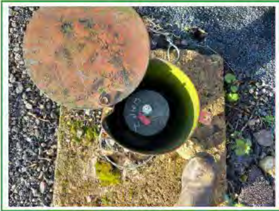
Photo No.14: Former gas monitoring point / borehole noted within Plot No.104 with bung and tap remaining insitu
