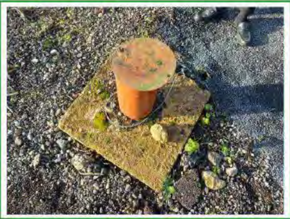
Photo No.13: Former gas monitoring point / borehole noted within Plot No.104
