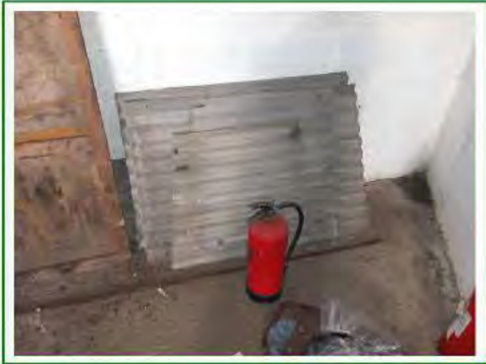
Photo No.71: PACM roofing / cladding noted stored within Unit No.16
