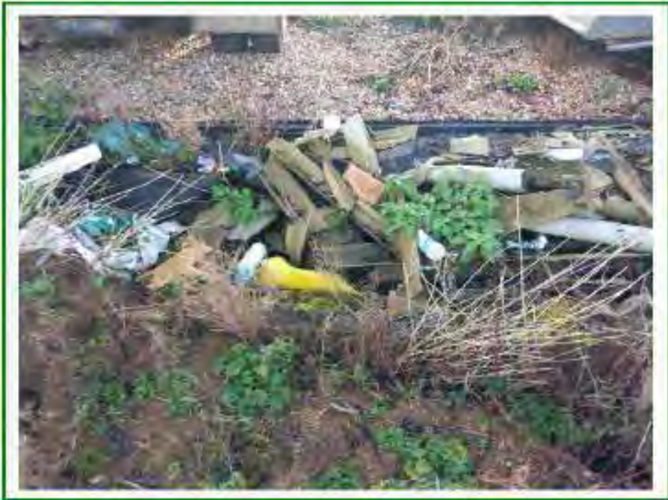
Photo No.23: Further shot of fragmented PACM, ash, debris and refuse between Plots No.105 & 106
