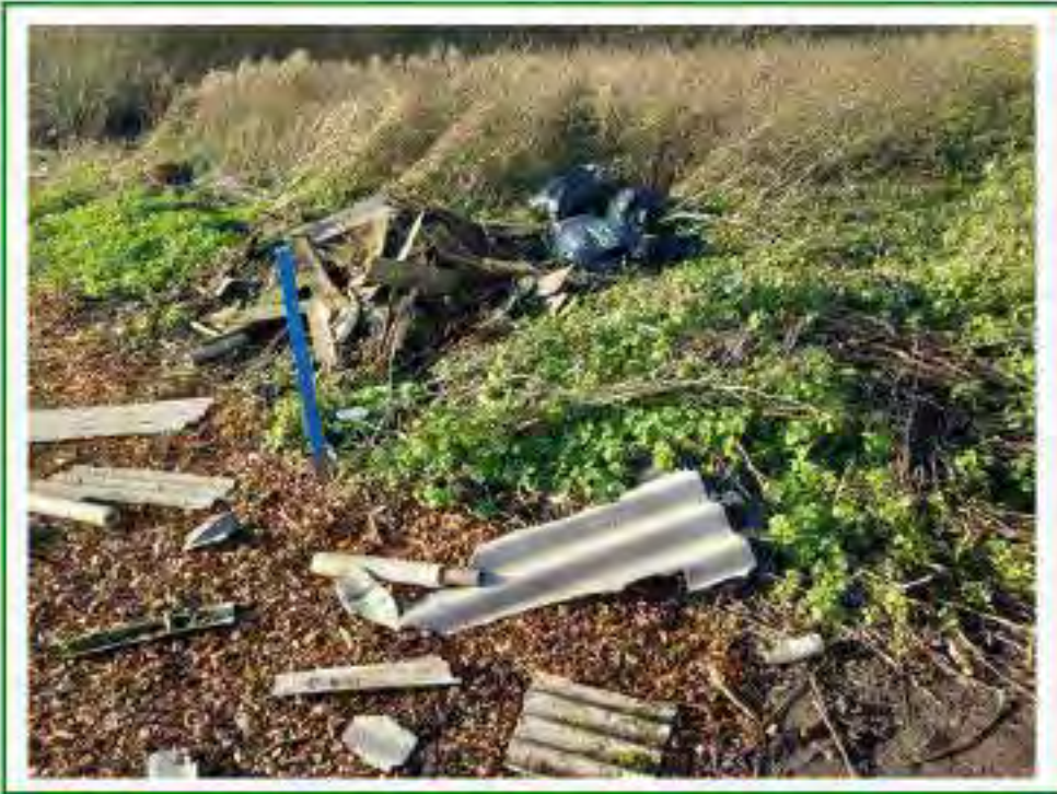
Photo No.3: Heap of fly-tipped debris and refuse including fragmented PACM adj. to the site access route
